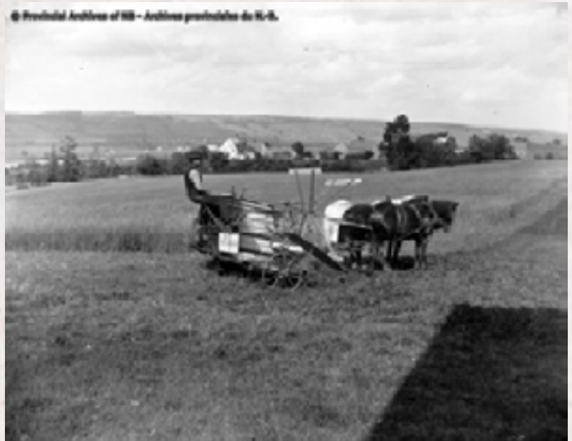
Horse-drawn binder (cuts wheat, oats, etc., and binds the stocks). Photograph courtesy of the Provincial Archives of New Brunswick, P5-100.
