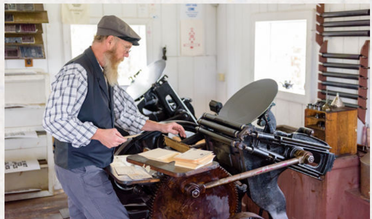
A printer operates the treadle platen press to print postcards.
